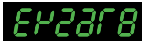
Example of Mirror Reverse display format displaying the number 876543
