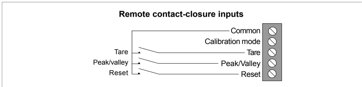
**CALIBRATION MODE** A contact closure which selects either direct or theoretical calibration method.
