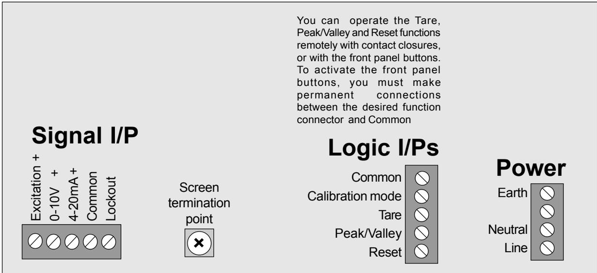
Use screened cable for the input signal and connect the screen to power earth at the meter end of the cable only. For best performance, keep the signal cable well away from the power and alarm cables, which could carry electrical noise likely to interfere with your measurement.
