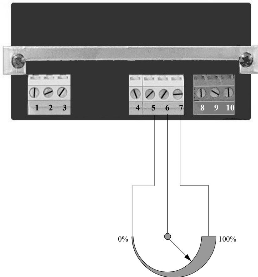
In this example, a 1Kilohm linear potentiometer allows you to adjust the brightness from 0% to 100 %
