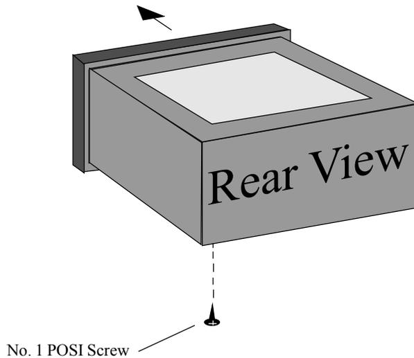
Withdraw the whole assembly from the front. Cut and solder links in new position, and replace assembly, screw and front cover.
