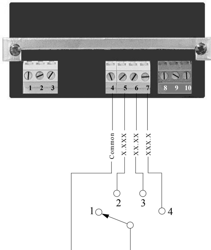
In this example, a 4 way rotary switch allows selection of 4 decimal point positions.
