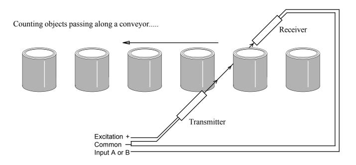
A through-beam system is often the most effective method of counting objects as they pass along a conveyor. The system relies on the containers breaking a light beam as they pass along the conveyor, and is quite insensitive to reflections, and does not rely on the surface colour or tint of the objects passing by.
