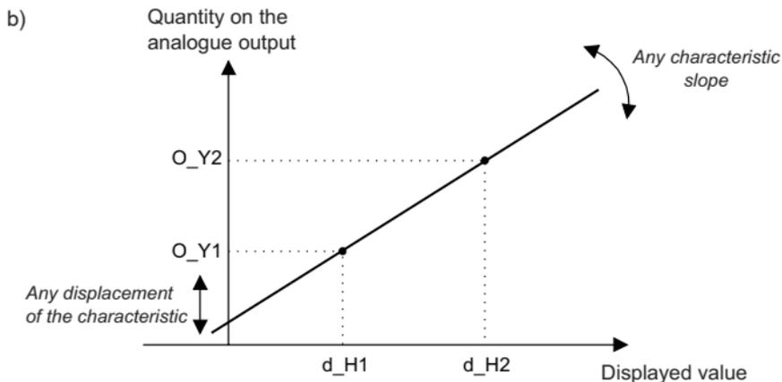
Value  $d_{H1}$  on the display => value  $O_{Y1}$  on the analogue output.
