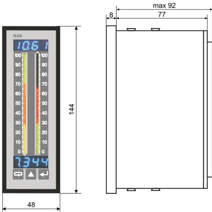
**Fig. 2. Meter overall dimension**
