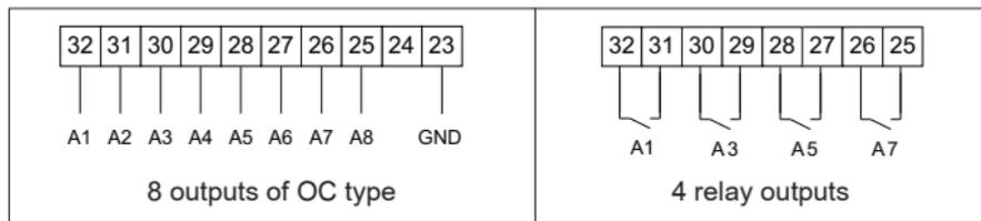
**c/ Connection way of digital and analogue output signals depending on the execution code**
